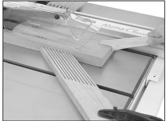
Figure 43. Typical ripping operation.
